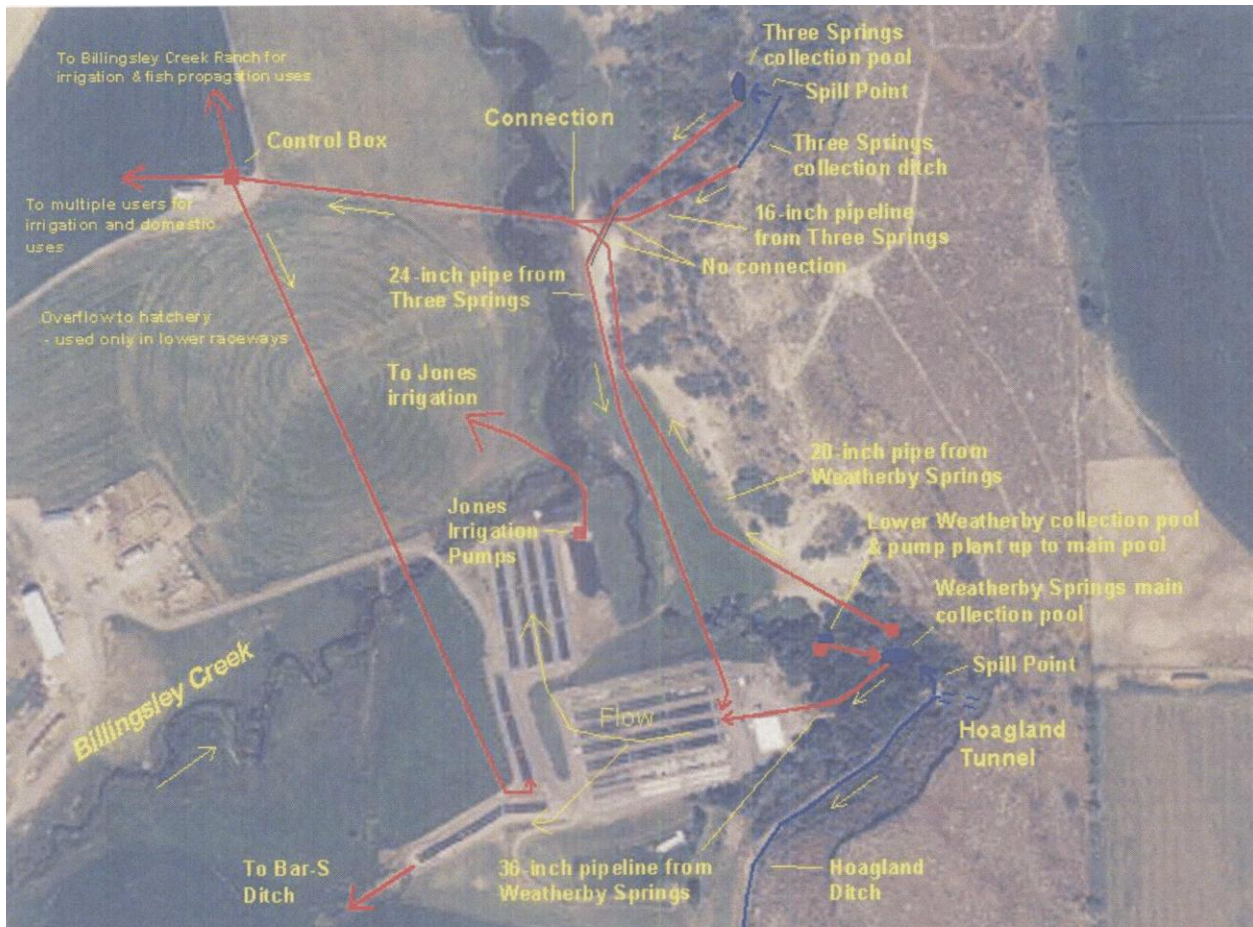
Figure 1. Conceptual layout of spring discharge collection and conveyance facilities from July 29, 2005 order 1 .
